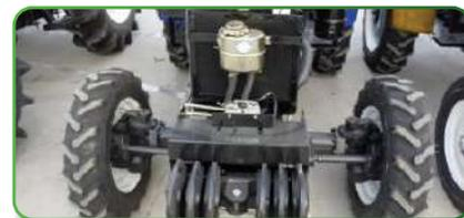
New designed front axle is adopted on 4WD tractor, mid hydraulic cylinder makes the structure easier and more reliable. The tie rod is canceled to provide higher clearance and better passing ability.
