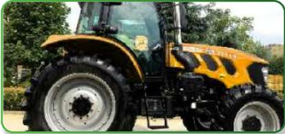
240 liters of double under-mounted fuel tanks, long continuous operation time and high operating efficiency. Full hydraulic steering system, easy to drive, flexible steering, front and rear adjustable steering wheel, more comfortable.
