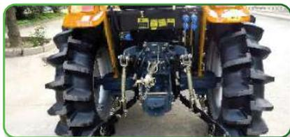
Equipped with international standard NTP 1/2 hydraulic output connectors, 1/2 way multi-valve and hydraulic pump with output flow of 35 l/m;
