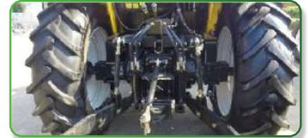
Double pressure hydraulic lifter, equipped with 325/328 gear pump; 3 sets of hydraulic multi-way valves are provided to meet the power requirements of various machines.
