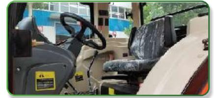
Using 16F+8R meshing shuttle type gear shift, reasonable speed matching, good working adaptability, optional crawler gear.
