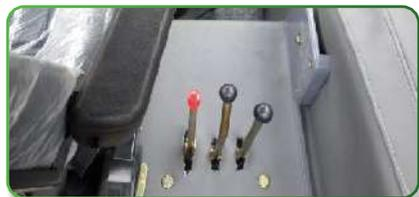
The use of flat floors, hanging pedals, side manipulation, 16+8 shuttle shift transmission, and various gear selections can provide a reasonable velocity distribution;
