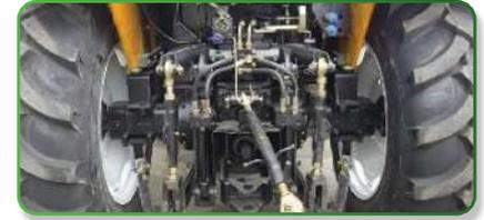
Comprehensive force/position control lifter for easy and convenient operation; strong pressure device lifter with up to 1800kg of max lifting force at the suspension point for the best rotary tillage and ploughing effect.
