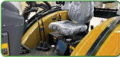
12F+12R shuttle-type gear shifting with quick forward and reverse has a variety of gear selection, and a reasonable velocity distribution;
