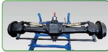
ZF(Germany) front axle is used on the tractor having high carrying capacity and clearance; double steering cylinders make the steering more flexible;
